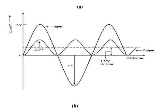
Fig. 3.13 (a) circuit diagram and (b) input -output waveform of frequency doubler
