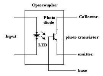
The LED phototransistor optocoupler shown in figure. An infrared LED acts as a light source and the phototransistor acts as a photo detector.
