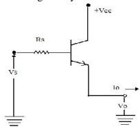
Fig.1.6 Voltage source circuit using Impedance transformation:
