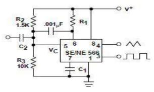
Fig. 3.19 External connections of VCO
