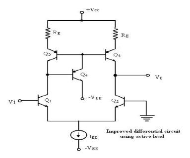
Fig.1.14. Improved differential circuit using active load
