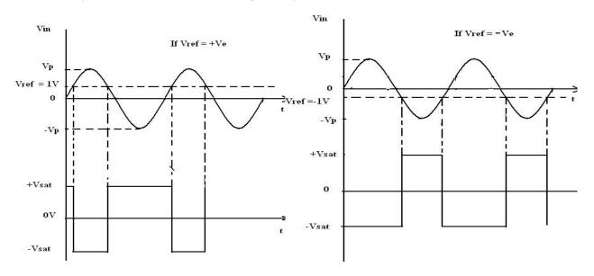
Input and Output Waveforms of non-inverting comparator
