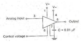
Fig.4.12 Connections of S&H IC
