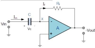
The input signal to the differentiator is applied to the capacitor. The capacitor blocks any DC content so there is no current flow to the amplifier summing point, X resulting in zero output voltage. The capacitor only allows AC type input voltage changes to pass through and whose frequency is dependant on the rate of change of the input signal.
