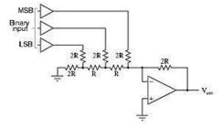
Fig.4.4 Ladder type DAC circuit
