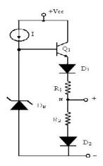
Fig.1.10 Voltage reference circuit using temperature compensation scheme
