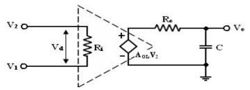
Fig 1.18 Equivalent circuit of practical circuit
