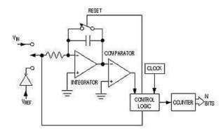
Fig 4.18 Sigma-delta ADCs/ Over sampling Converters:
