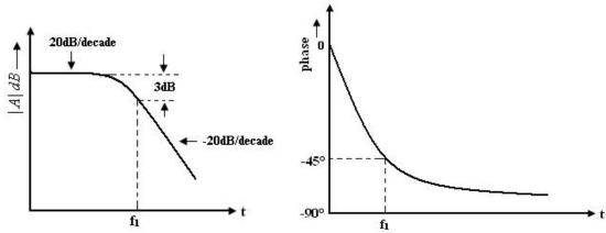
Fig 1.19 Frequency response of op amp
