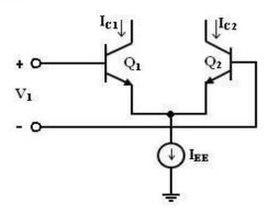
Fig.3.5 multiplier circuit using an emitter coupled pair
