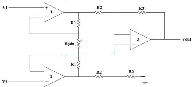
A Typical Three Op-amp Instrumentation Amplifier
