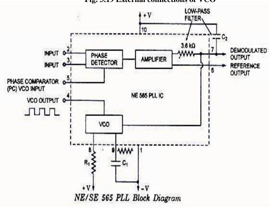
The center frequency of the PLL is determined by the free running frequency of the VCO, which is given by
