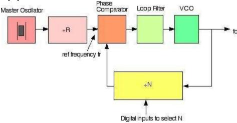
Fig. 2.24 PLL based frequency synthesizer
