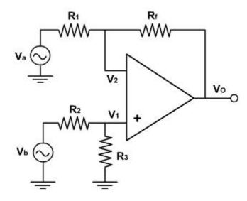
Since there are two inputs superposition theorem can be used to find the output voltage. When  $V_b = 0$ , then the circuit becomes inverting amplifier, hence the output due to  $V_a$  only is
