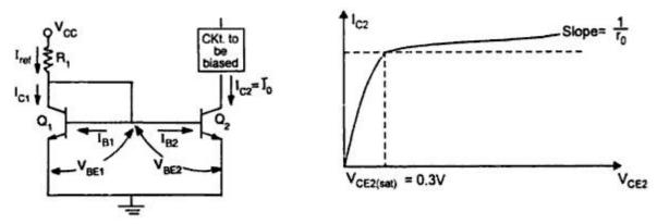
Fig. 1.1 Current mirror circuit Fig 1.2 Current source output current characteristics
