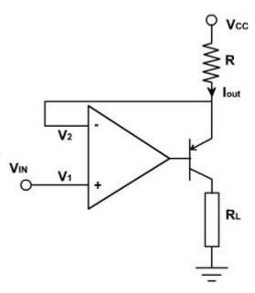
In this circuit, because of negative feedback  $V_{BE}$  is automatically adjusted. For instance, if the load resistance decreases the load current tries to increase. This means that more voltage is feedback to the inverting input, which decreases  $V_{BE}$  just enough to almost completely nullify the attempted increase in load current. From the output current expression it is clear that as  $V_{in}$  increases the load current decreases.
