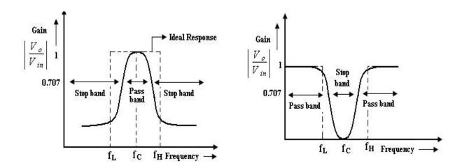
Frequency response of Band Pass filter and Band reject Filter
