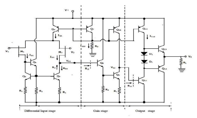
Fig. 1.17 Internal stages of Op-amp Output stage:
