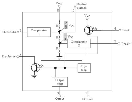
From the above figure, three 5k internal resistors act as voltage divider providing bias voltage of 2/3 Vcc to the upper comparator & 1/3 Vcc to the lower comparator. It is possible to vary time electronically by applying a modulation voltage to the control voltage input terminal (5).
