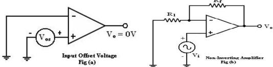
Let us determine the  $V_{OS}$  on the output of inverting and non-inverting amplifier. If Vi = 0 (Fig (b)
