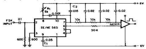
Fig. 3.21 FSK demodulator circuit
