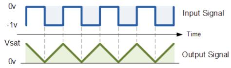
We know from first principals that the voltage on the plates of a capacitor is equal to the charge on the capacitor divided by its capacitance giving Q/C. Then the voltage across the capacitor is output Vout therefore: -Vout = Q/C. If the capacitor is charging and discharging, the rate of charge of voltage across the capacitor is given as:
