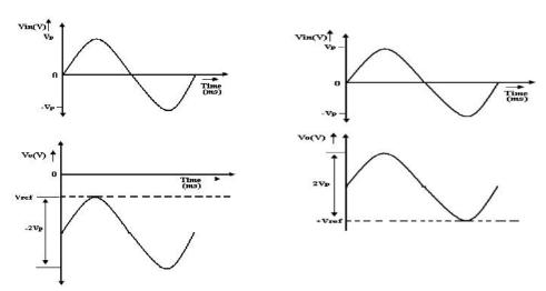
Input and Output Waveform with -Vref
