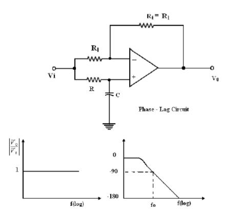
The relationship is complex as defined above equation and it shows that it has both magnitude and phase. Since the numerator and denominator are complex conjugates, their magnitudes are identical and the overall phase angle equals the angle of numerator less the angle of the denominator.
