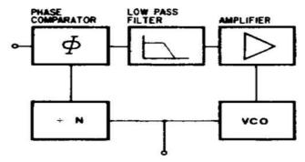
The circuit of the figure above can also be used for frequency division. Since the VCOoutput (a square wave) is rich in harmonics, it is possible to lock the m-th harmonic of the VCO output with the input signal fs. The output fo of VCO is now given by fo=fs/m
