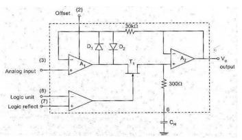
Fig.4.11 LF 398 IC-Functional Diagram
