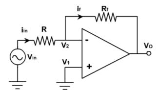
Assuming OPAMP to be an ideal one, the differential input voltage is zero.
