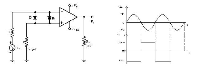
Zero crossing detector circuit and input-output waveforms
