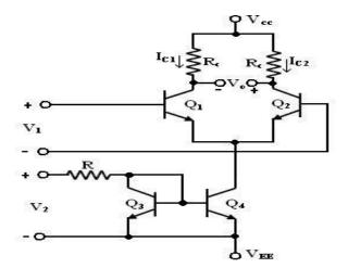
Fig. 3.7 A simple modulator using a differential amplifier
