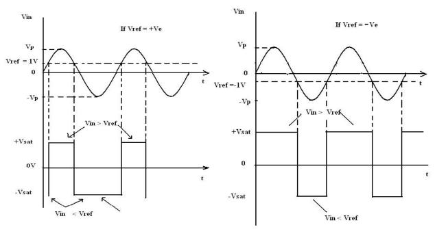
Input and Output Waveforms of non-inverting comparator
