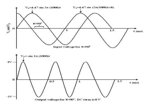
Fig. 3.16 input- output waveforms of phase angle detector 3.5 Operation of Basic Phase Locked Loop
