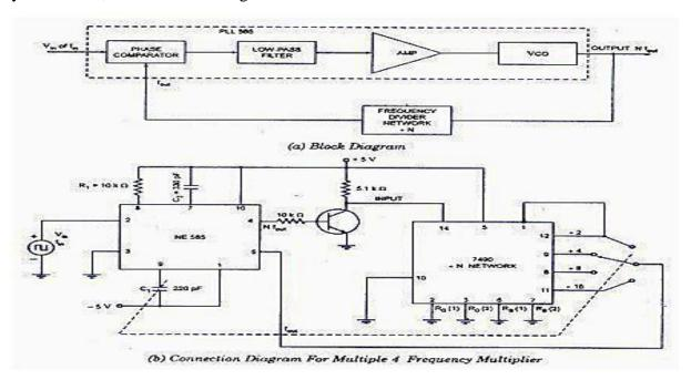
Fig. 3.20 Frequency multiplier using PLL
