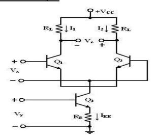
Fig. 3.9 Differential stage of the Tran conductance multiplier
