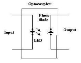
LED photodiode shown in figure, here the infrared LED acts as a light source & photodiode is used as a detector.
