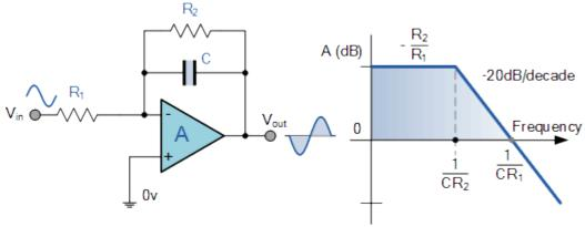
Unlike the DC integrator amplifier above whose output voltage at any instant will be the integral of a waveform so that when the input is a square wave, the output waveform will be triangular. For an AC integrator, a sinusoidal input waveform will produce another sine wave as its output which will be 90° out-of-phase with the input producing a cosine wave.
