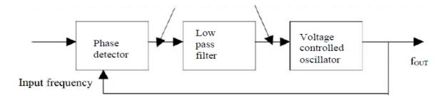
Fig 3.17 Block diagram of PLL
