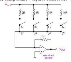
Fig. 4.3 weighted resistor DAC using Op-amp
