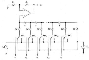
Fig. 4.6 Voltage mode DAC
