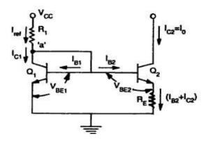
Fig.1.3 Simple current source
