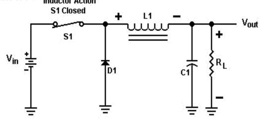
As we see above, L1, which tends to oppose the rising current, begins to generate an electromagnetic field in its core. Notice that diode D1 is reversed biased and is essentially an open circuit at this point. Now lets take a look at what happens when S1 opens below:
