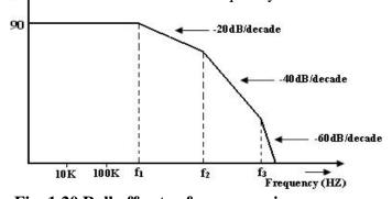
Fig. 1.20 Roll off rate of op amp gain
