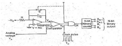
Fig. 4.16 A/D Using Voltage to Time Conversion:
