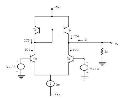
Fig. 1.13 BJT differential amplifier with current mirror active load Analysis of BJT differential amplifier with active load:
