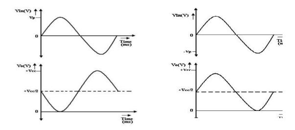
Input and output waveform with +Vref
