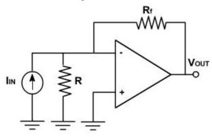
Due to virtual ground the current through R is zero and the input current flows through  $R_{\rm f}$ . Therefore,  $v_{out}$  =- $R_{\rm f}$  \*  $i_{\rm in}$
