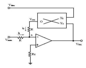
Fig 3.14 divider circuit
