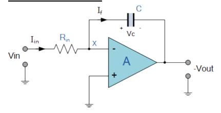
As its name implies, the Op-amp Integrator is an operational amplifier circuit that performs the mathematical operation of Integration, that is we can cause the output to respond to changes in the input voltage over time as the op-amp integrator produces *an* output voltage which is proportional to the integral of the input voltage.
