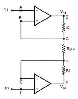
Input Stage of Instrumentation Amplifier
