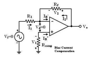
Fig. 1.22 Bias compensated circuit
