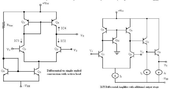
Fig.1.15. Differential to single ended conversion and output stage Differential Mode signal analysis:
