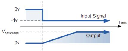
The rate at which the output voltage increases (the rate of change) is determined by the value of the resistor and the capacitor, "RC time constant". By changing this RC time constant value, either by changing the value of the Capacitor, C or the Resistor, R, the time in which it takes the output voltage to reach saturation can also be changed for example.
