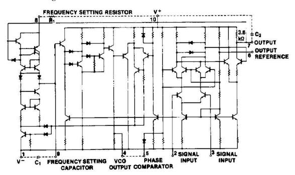
When PLL is locked to an input frequency, the error voltage vc(t) is proportional to (fs-fo). If the input frequency is varied as in the case of FM signal vc will also vary in order to maintain the lock. Thus the voltage output serves as a frequency discriminator which converts the input frequency changes to voltage changes.
