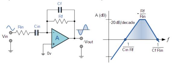
Adding the input resistor  $R_{IN}$  limits the differentiators increase in gain at a ratio of  $Rf/R_{IN}$ The circuit now acts like a differentiator amplifier at low frequencies and an amplifier with resistive feedback at high frequencies giving much better noise rejection.
