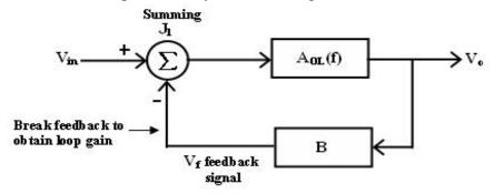
Fig. 1.21 Feedback loop system
