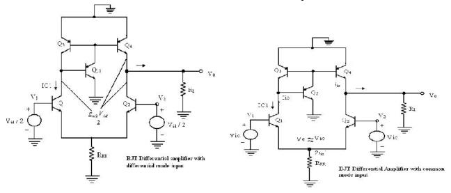
Fig. 1.16 Differential amplifier with differential mode input and common mode input 1.6 Basic information about operational amplifiers
